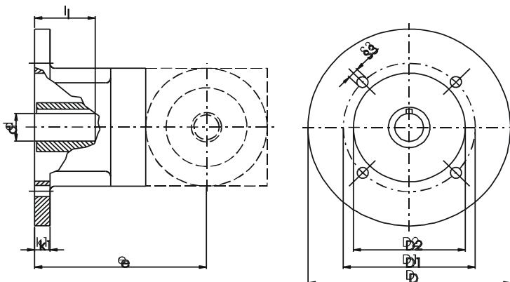
All types of bevel gears are available ready for motor mounting or in combination with three-phase motors. The type with mounted motor features a flange bearing neck on side 3 of the gear (see picture) instead of a bearing neck. Please refer to the following table for the dimensions. All other dimensions can be found next to the respective gear type.
