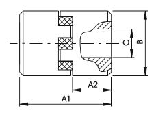
The couplings are torsionally elastic, transmit the torque positively and are puncture-proof.
